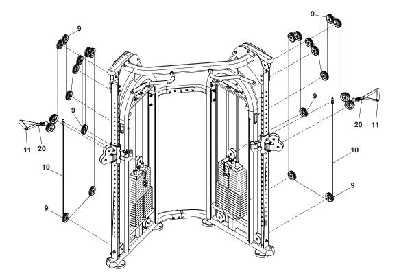
**NOTE:** The weight cables (10) are installed in a similar manner for both the left weight stack frame (1) and the right weight stack frame (2).
