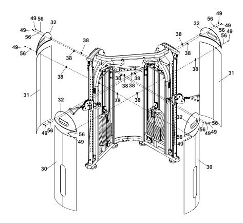
**NOTE:** Shrouds are installed in a similar manner for both the left weight stack frame (1) and the right weight stack frame (2).
