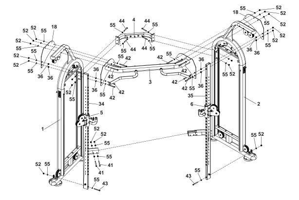
Align the lower coupling on the right weight stack frame (2) with the receptacle on the left weight stack frame and slide the coupling into the receptacle, aligning the drilled holes.
