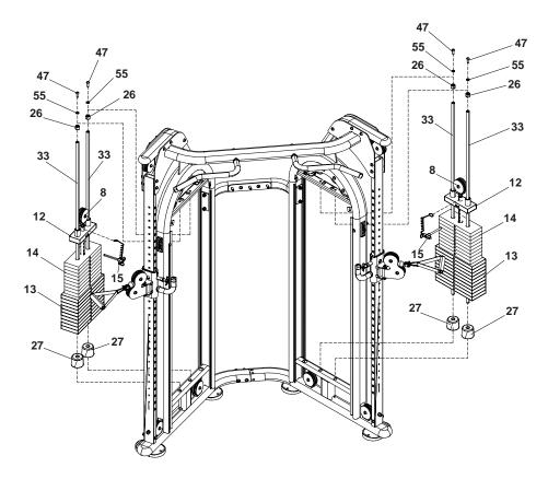
**NOTE:** Weight stacks are assembled in a similar manner for both the left weight stack frame (1) and the right weight stack frame (2).
